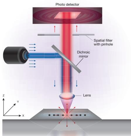
Figure 1. A simplified view of confocal microscopy.
